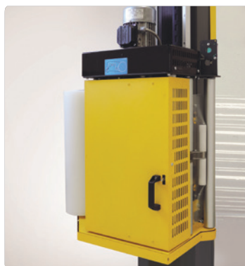
LP - Powered pre-stretch 240% (200% - kit available as option)
